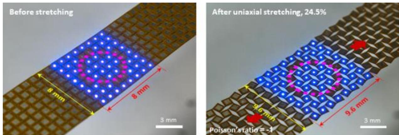
Description: When the meta-display is stretched lengthwise, it is also stretched widthwise at the same ratio, so that the displayed image can be expanded without distortion.
