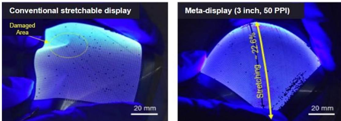
Description: A 3-inch meta-display and a conventional stretchable display are attached to a hemispherical surface with a radius of 80 cm. The conventional stretchable display shows wrinkles and creases occur, but the meta-display is attached smoothly without any damage.
