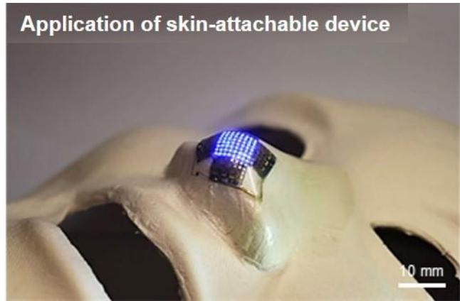
Description: The manufacturing of curved displays that use meta-displays to display images and devices that can be attached to the skin.
