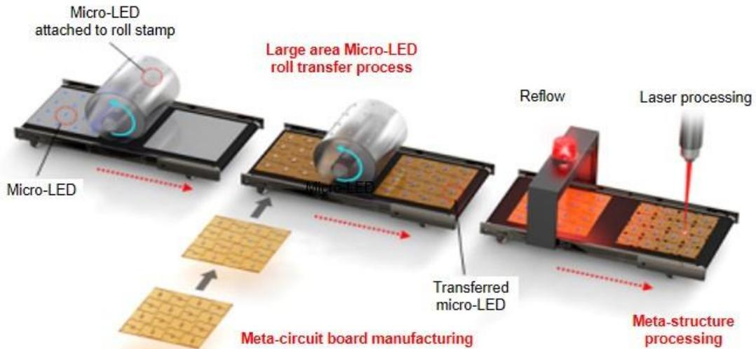
Description: A meta-display can be manufactured by transferring a micro-LED device to a large-area meta-circuit board using roll-based large-area transfer technology. After micro-LED transfer, the meta-display is manufactured through reflow and meta-structure processing using a laser.
