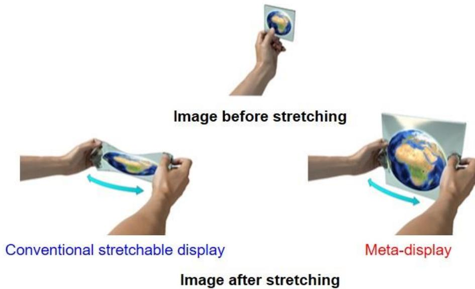
Description: When stretched lengthwise, the conventional stretchable display shrinks widthwise, resulting in the distortion of the displayed image. However, since the meta-display stretches at the same ratio widthwise when stretched lengthwise, it is possible to stretch the display without any image distortion.
