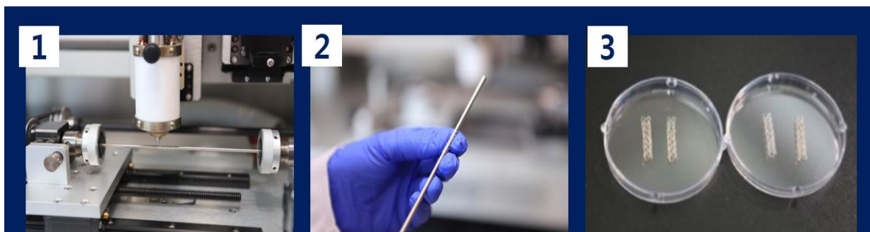
Photo: ①② Production of a stent using bio 3D printer / ③ Samples of biodegradable polymer stents
