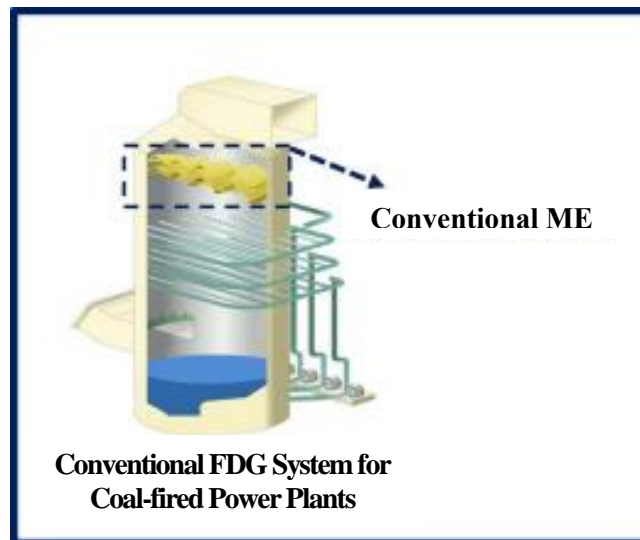
Picture 1: At the chimneys of coal-fired power plants, Flue Gas Desulfurizers (FGD) are installed; the Mist Eliminator (ME) is installed on top of the FGD, to reduce the fine dust. Picture 1 shows the design of a ME using the inertial impaction method, which is used at 90% of domestic coal-fired power plants.
